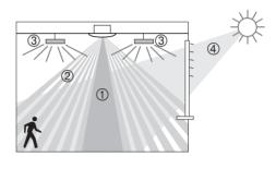
① Mixed light measurement② Motion detection
