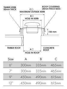
In addition to the size 6, 7, 9 & 12 Roof Termination Sets, the Roof Plate Assemblies can also be used with the following Roof Terminations part numbers.
