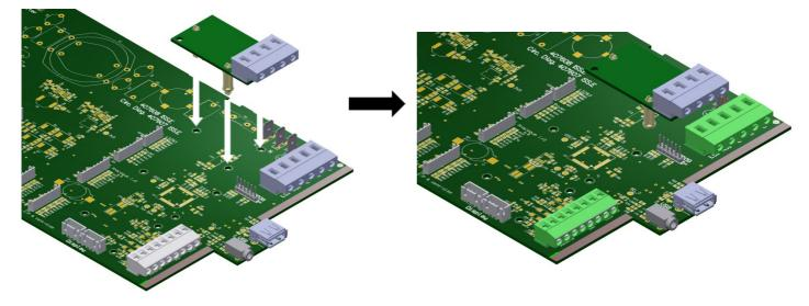
4. Connect the lead from LS2/3 PCB into the socket J21 shown below.
