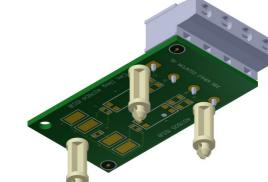
3. Fit the LS2/3 PCB to the main PCB in position shown.
