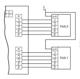
NOTE: 3 PHASE FANS MUST HAVE EXTERNALLY CONNECTED THERMAL OVERLOAD PROTECTION.
