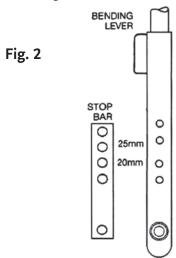
3. Remove the bending lever locking pin 2 from hole 2 (see Fig. 1); ensure the grooved roller is fitted in the correct position (Fig. 2) for the conduit being formed.
