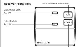
Learn button enabling communication between the transmitter and receiver, also control button for output in manual mode
