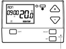
Press the Reset button located beneath the drop down flap
