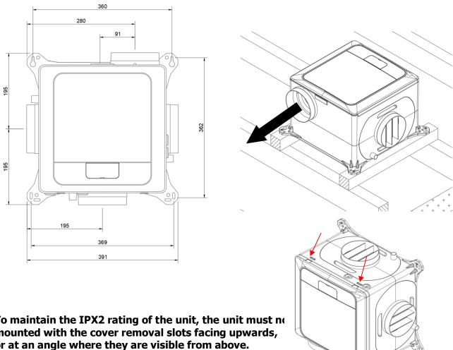
To maintain the IPX2 rating of the unit, the unit must no mounted with the cover removal slots facing upwards, or at an angle where they are visible from above. All other orientations are acceptable.
