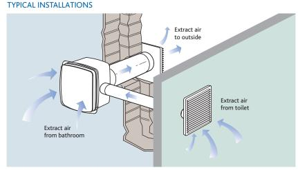
Typical installation of fan unit with optional subsidiary spigot kit in bathroom and adjacent toilet application.
