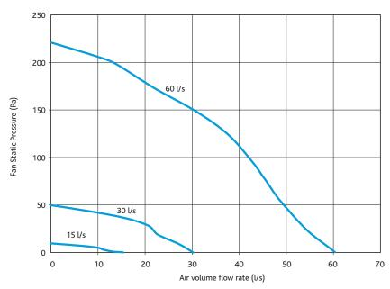
Graphs above includes 300mm duct and low resistance wall grille.
