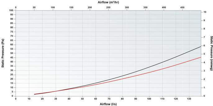
1 x Filter housing (CW-F 520) with 2 x 180 mm end plates (CW-P 520) and filter (CW-F9 520)
