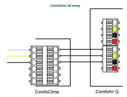
3 core cable, 1.5mm Max. (up to 50 metres)
