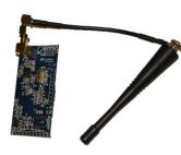
The Zehnder RF-PCB enables the CCRFZ (655 000 755) controller to be used with the ventilation system without the need for the ComfoSense C67.
