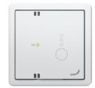
The Zehnder 12V 0-10V remote CO2 sensor and combined three position switch is designed to enable the user to manually select the desired ventilation systems flow rate based on the visual air quality indicator, or automatically adjust the unit relevant to the CO2 level.
