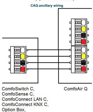
4 core cable, 1.5mm Max. (up to 50 metres)
