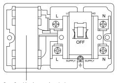
Fuse Cartridge (remove by gripping and pulling up and away from the fuse cartridge holder)
