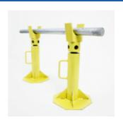
The Termination Technology range of cable jacks are suitable for lifting large drums of cable off the ground for easy reeling. Mechanical screw type operation with two jacks and a spindle bar. The Base plates on the jacks are designed to give stability even on soft ground. Available in 3 tonne, 6 tonne and 8 tonne versions.
