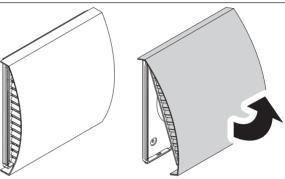
4. Fix the back wall of the ventilation hood on the wall using the supplied screws 4x40.
