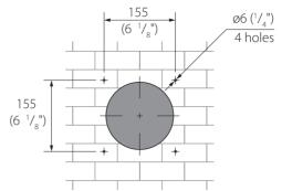
3. Insert the supplied expansion anchors 6x40 into the holes. Disassemble the outer ventilation hood to enable access to the fastening holes.
