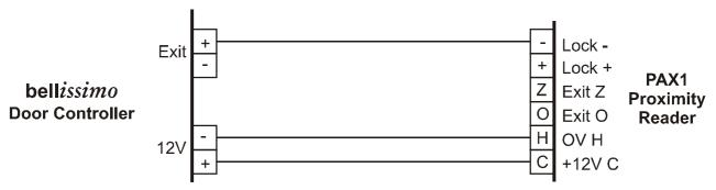
Connect the lock release as per this manual. Leave the Proximity Reader set to fail secure, the BSD controller sets the lock type.
