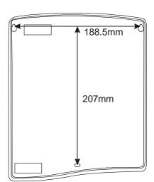
screw to be inserted at the bottom. Tighten all three screws. Before replacing the Front Cover remove the protective film from the display lens and also check that the DipSwitch settings are correct or change as necessary (see Page 22).
