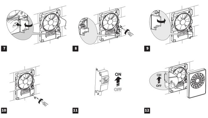
The fan is suitable for mounting anywhere outside of Zones 1 or 2 of your wetroom. The fan may be connected to power mains by four wiring diagrams. The fan is compatible with 100-240 V / 50-60 Hz power mains. The Aura Smart MSHT has Li terminal for connection to the lamp up to 200W/230 V or 100 W/120 V. At this connection the fan will be switched on signal from the motion sensor.
