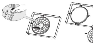
The fan casing has three round lowered tabs for cable entry. Cut out a hole at the most suitable place with a knife.
