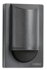
Attractive, clever, efficient. Infrared motion detector IS 2180-2 for outdoors, ideal for building fronts and properties, medium-sized business and outdoor spaces, ideal installation height 2 m, 180° angle of coverage, reach. 12 m max. or 5 m max. (tangential), selectable time and twilight threshold, manual override, including corner wall mount for external and internal corner.
