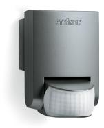
Targeted detection all around the building. Infrared motion detector IS 130-2, for indoors and out, ideal for targeted detection close to the building, 130° angle of coverage, reach up to 12 m, selectable time and twilight threshold, sensor turns through 50° and tilts through 90° for exact adjustment of the detection zone.
