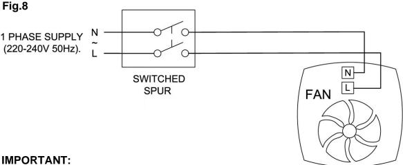
In order to have the product switch off in the event of a fire it must be wired using a smoke alarm with a relay system.
