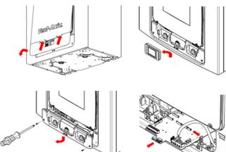
2. Fit the three plastic stand-offs provided, into the three holes in the Input Switch PCB.
