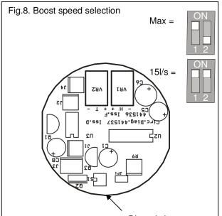
**Max speed boost:** Dip switch 2 in the 'OFF' position.
