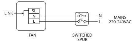
Fig.2 Continuous Boost (15 L/s) with no trickle facility. Note:- Link must be fitted between Live & Switched Live terminals.
